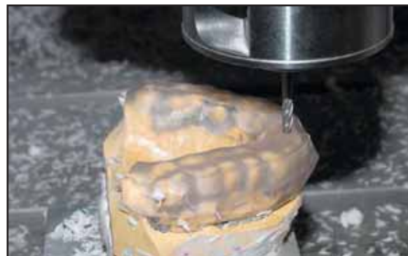
Fig. 7 Acrylic splint mounted in vertical machining center to remove excess material.
